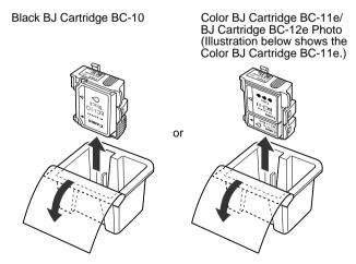
**8.** If you are installing a new BJ Cartridge, remove the orange protective cap and orange protective tape from the BJ Cartridge.
